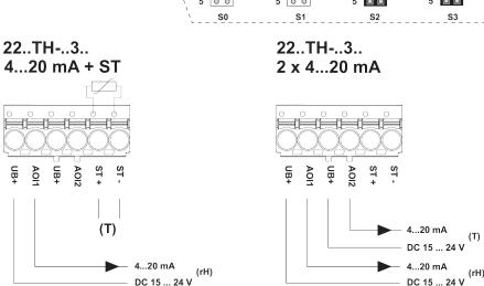
Connectors ST+ / ST- are only used for sensor types which additionally have a passive resistance sensor element for temperature measurement.
