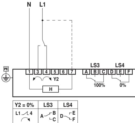
H: Internal heating (no need to connect internal heating for indoor applications with constant temperature conditions)
