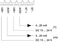
Connectors ST+ / ST- are only used for sensor types which additionally have a passive resistance sensor element for temperature measurement.
