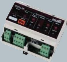
UK24-LON interface module is a second option to a LON configured actuator. This gateway allows the use of standard MFT actuators which connect to the gateway and communicates to the controller. Each UK24-LON can connect up to eight MFT actuators offering an economical solution.
