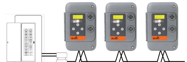
→ Peer to peer communication allows daisy-chain installation of up to 32 devices, reducing cabling.
