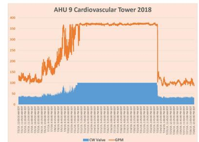
One of the AHUs maxed out at around 130 gpm. When the flow unexpectedly increased to nearly 400 gpm, it was evident that something in the system was performing poorly. Although a damaged and/or fouled coil was suspected, an inspection revealed that the culprit was actually a malfunctioning discharge air temperature sensor.
