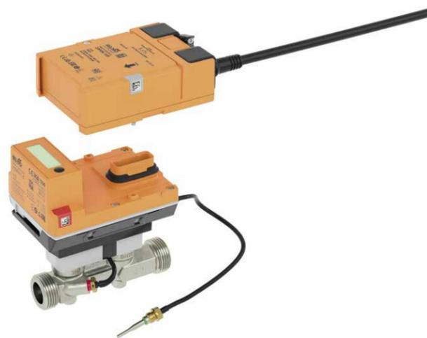
**Figure 46:** All wiring is to the logic module, allowing the MID / EN 1434 sensor module to be re-calibrated without disturbing the wiring.
