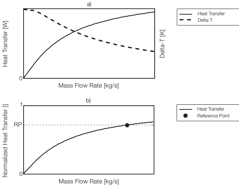
Figure 1: (a) Absolute and (b) normalized heat transfer capacity at design conditions. (The dip in the upper left corner of (a) is due to flow regime transition)
