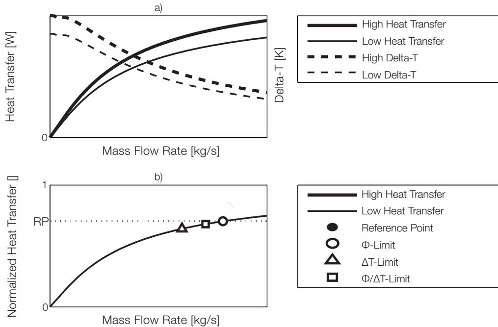
Figure 2: (a) Absolute and (b) normalized heat transfer capacity with flow, delta-T and flow/delta-T limiting results, assuming a 2K increase in chilled water supply temperature from 6 to 8°C.
