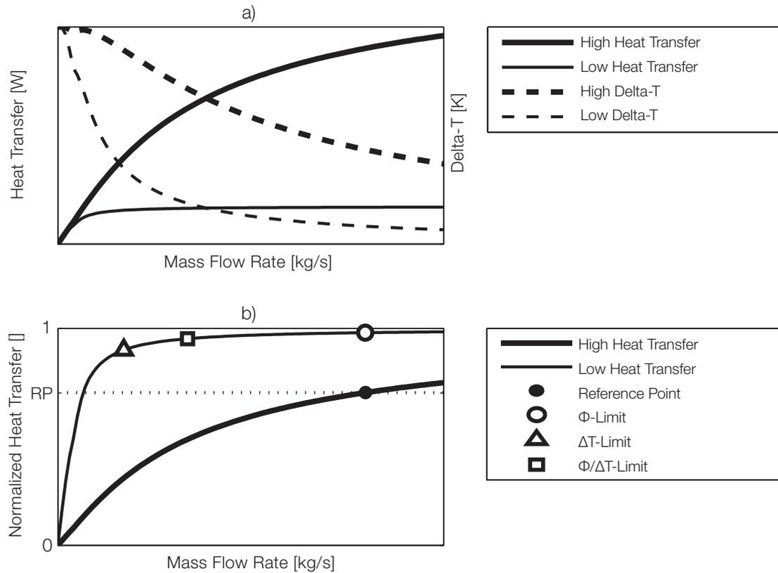
Figure 3: (a) Absolute and (b) normalized heat transfer capacity with flow, delta-T and flow/delta-T limiting results, assuming a factor 6 reduction in mass air flow rate.
