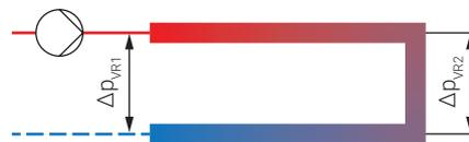
The constant flow that flows through the consumer is determined by the internal pump. The 3-way-Belimo Energy Valve™ only influences the mixing behaviour of the flow/bypass. The valve position is used to influence the quantity of return water that is added to the supply via the bypass.
