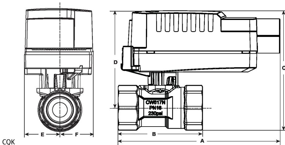
On/Off, Floating point, Non fail-safe, 24 V
