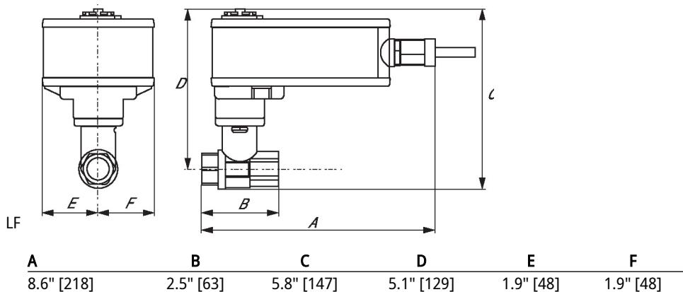
On/Off, Floating point, Non fail-safe, 24 V
