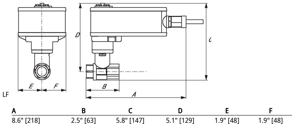
On/Off, Floating point, Non fail-safe, 24 V
