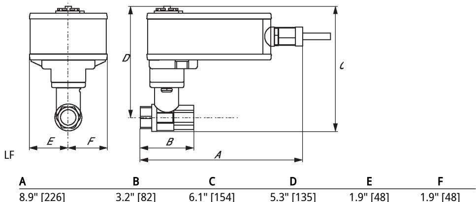
On/Off, Floating point, Non fail-safe, 24 V
