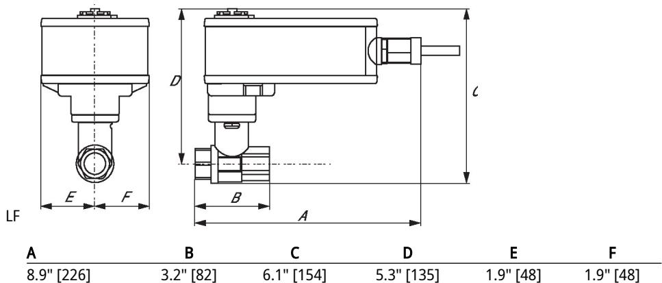
On/Off, Floating point, Non fail-safe, 24 V
