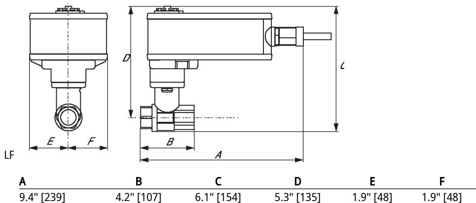
On/Off, Floating point, Non fail-safe, 24 V
