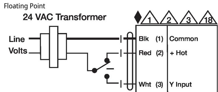
**24 VAC Transformer**
