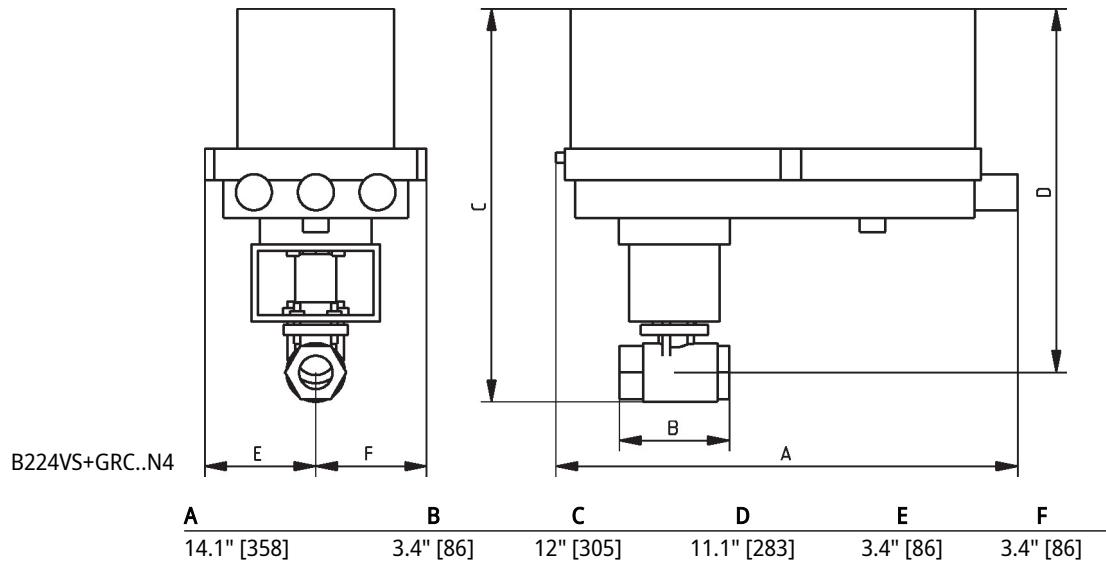
On/Off, Floating point, Non fail-safe, 24 V
