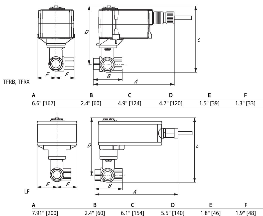
The technical drawings illustrate the dimensions of two BELIMO actuators: TFRB and LF. The top row shows the TFRB model, and the bottom row shows the LF model. Each row contains a front view on the left and a side view on the right. The side view indicates height dimensions D and C, width dimension A, and depth dimension B. The front view indicates width dimensions E and F. Below each row is a table listing these dimensions in inches and millimeters.
