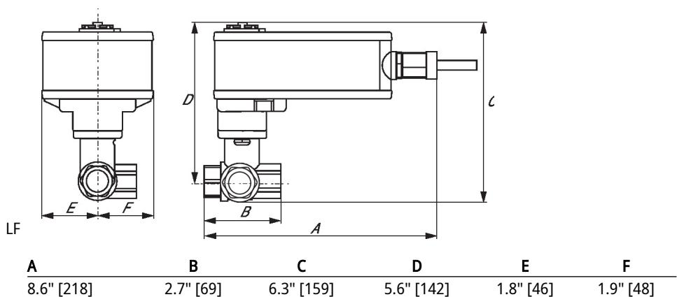
On/Off, Floating point, Non fail-safe, 100...240 V
