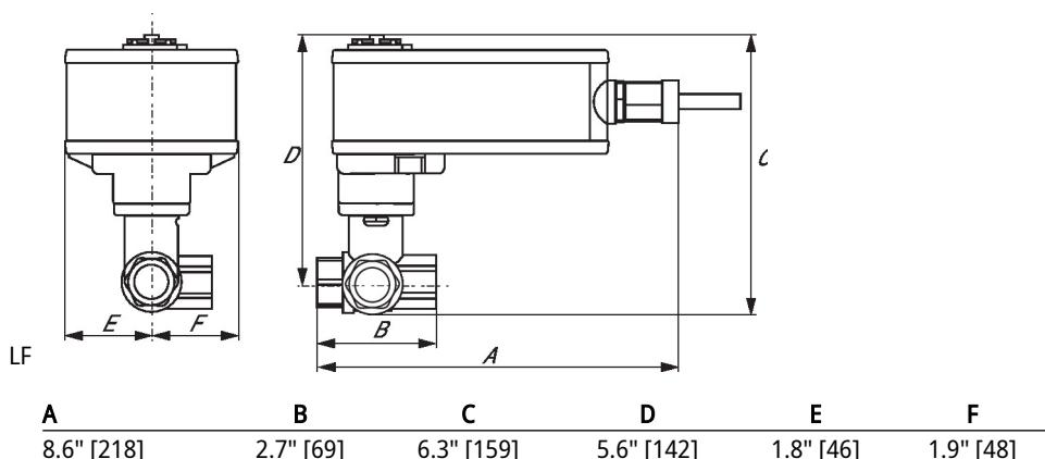
On/Off, Floating point, Non fail-safe, 24 V
