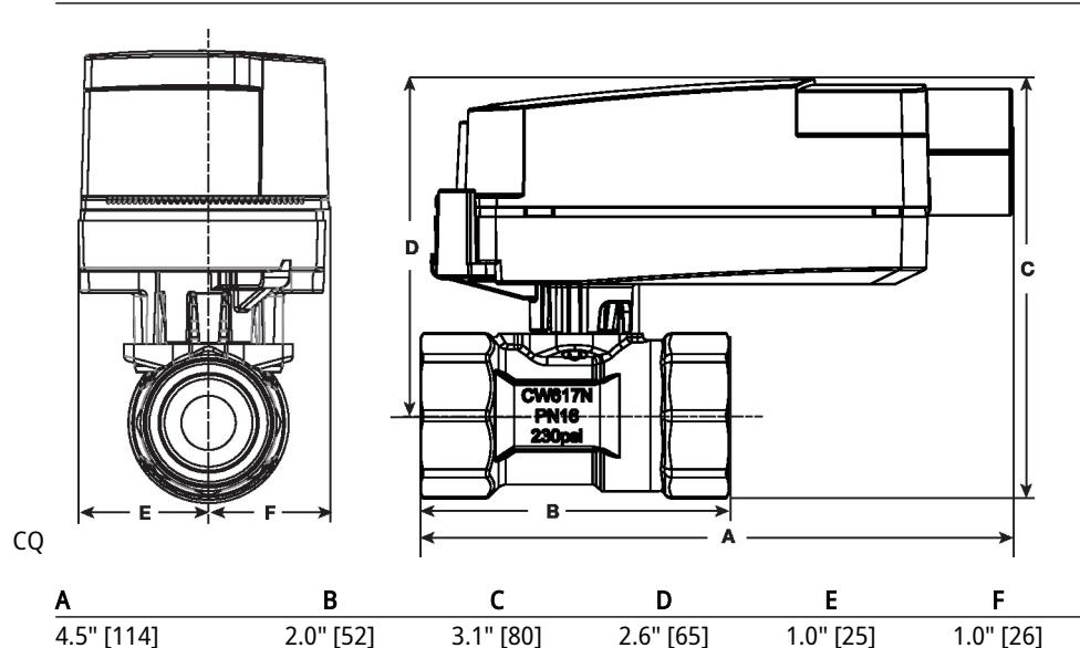
On/Off, Electrical fail-safe, 24 V
