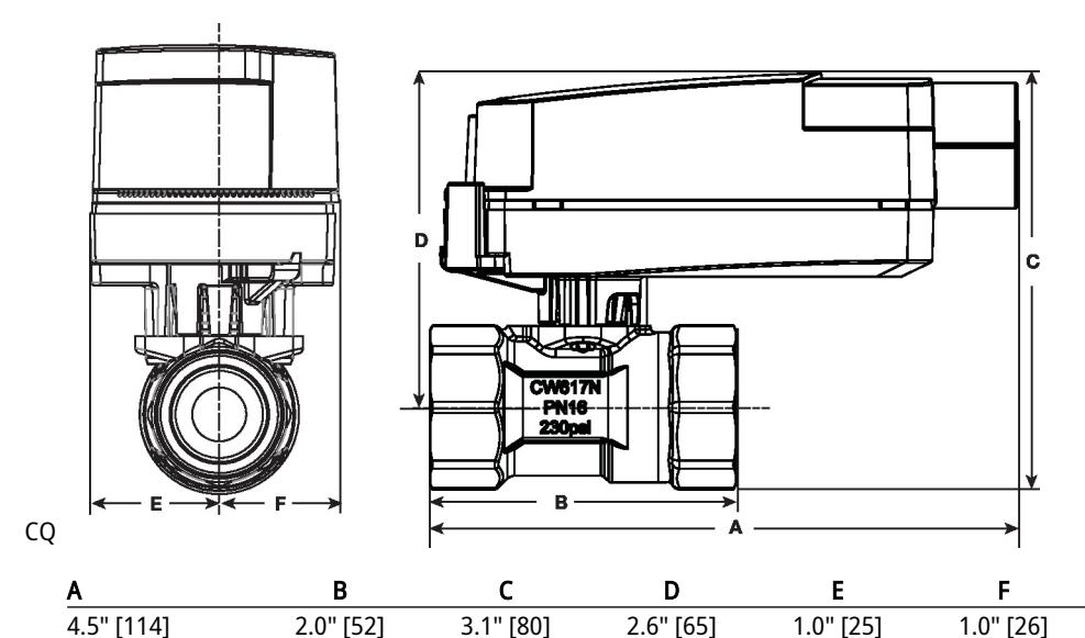
Modulating, Electronic fail-safe, 24 V
