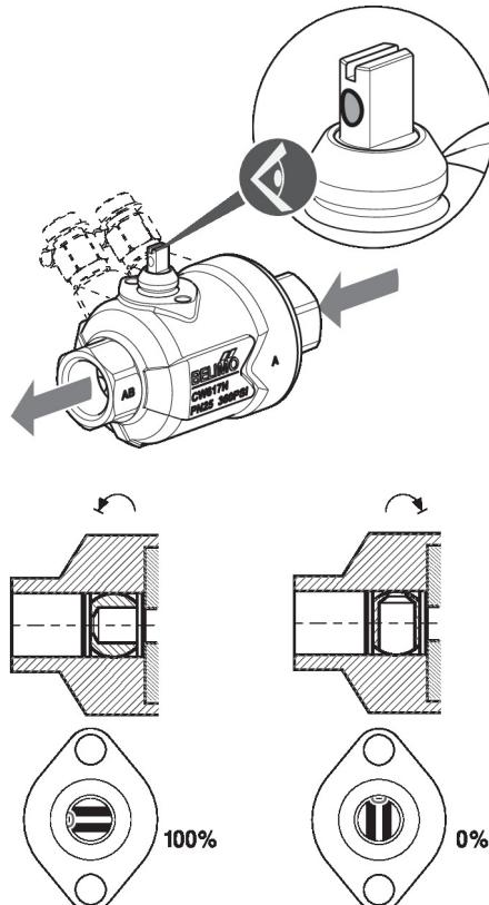
**Flow setting** The angle of rotation of the CQ.. actuator can be changed by end stop clip in 2.5° increments. This is used to set the V'max value (maximum flow rate of the valve).
