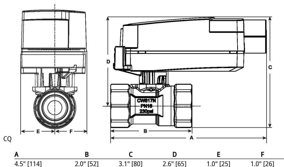
Modulating, Electronic fail-safe, 24 V
