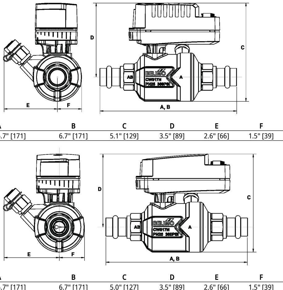
On/Off, Electrical fail-safe, 24 V
