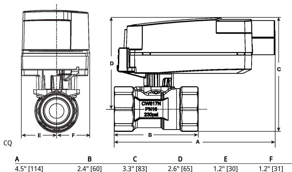
On/Off, Floating point, Non fail-safe, 24 V
