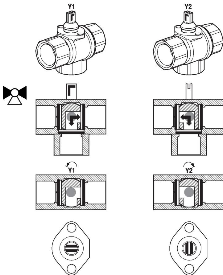
**Flow setting** At the actuator the end stop clip has to be removed in order to get the angle of rotation of 90°, which is needed for the change-over functionality.
