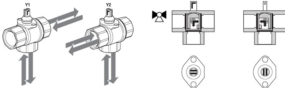
**Operating mode** The change-over zone valve is adjusted by a rotary actuator. The rotary actuator is controlled by an on/off signal.
