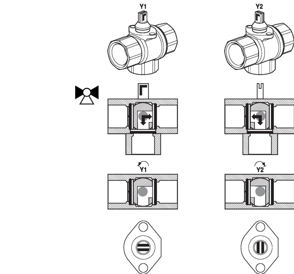
**Flow setting** At the actuator the end stop clip has to be removed in order to get the angle of rotation of 90°, which is needed for the change-over functionality.
