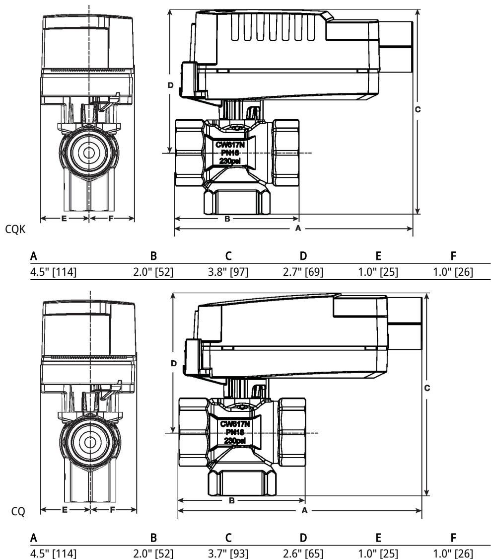
The technical drawings illustrate the dimensions of the Z3050QS-E actuator. The front view shows the actuator body with a flange and a central valve assembly. The side view shows the actuator body, a CW617N PN16 230psi valve, and the mounting flange. Dimension lines A, B, C, D, E, and F are indicated for each view.
