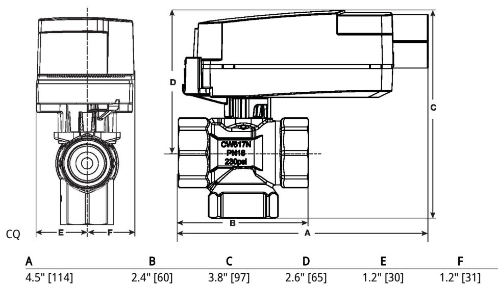
On/Off, Electrical fail-safe, 24 V
