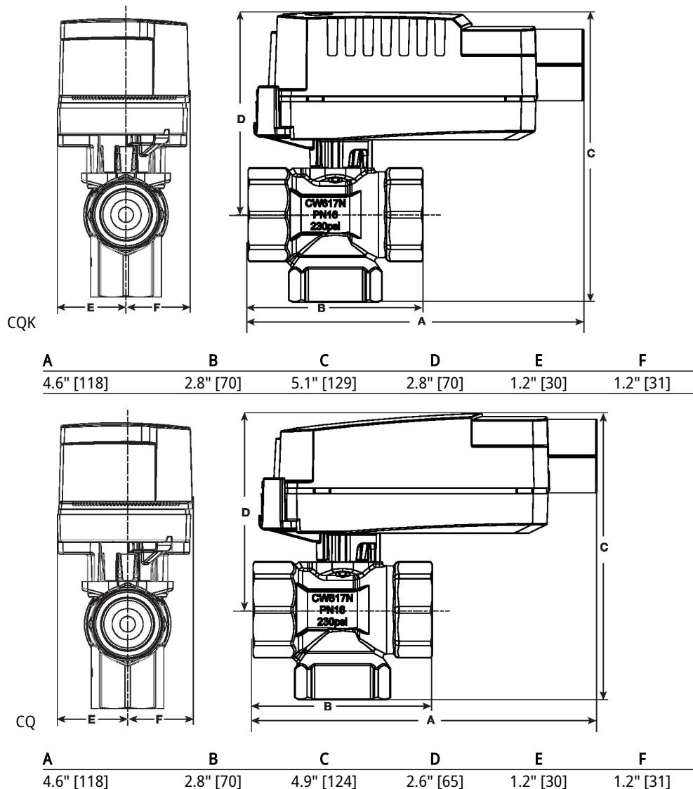
On/Off, Floating point, Non fail-safe, 100...240 V
