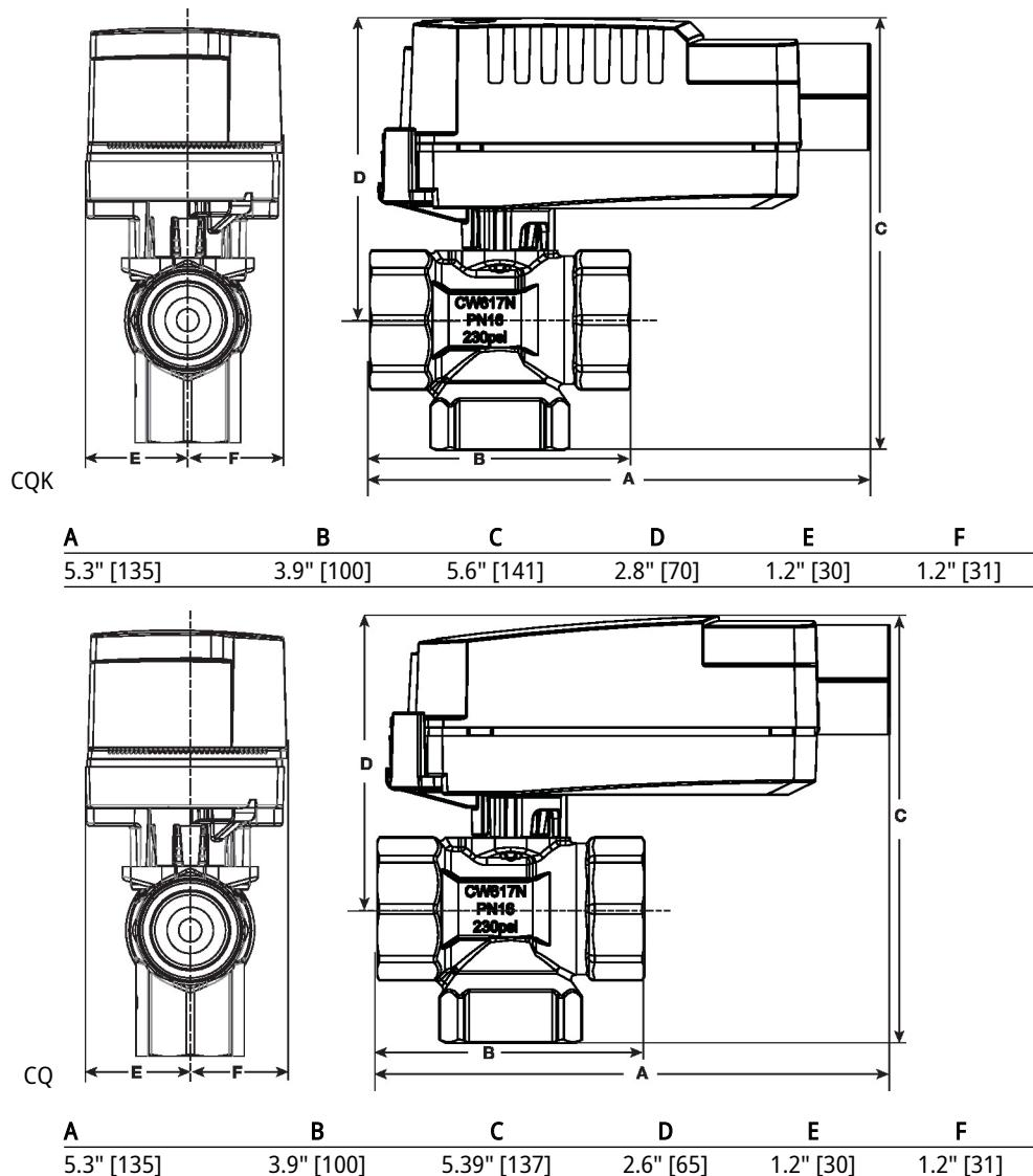
The technical drawings illustrate the dimensions of the Z3100QS-J actuator. The front view shows the actuator body with a flange and a central valve assembly. The side view shows the actuator body, a CW617N valve, and a flange. Dimension lines A, B, C, D, E, and F are indicated for each view.
