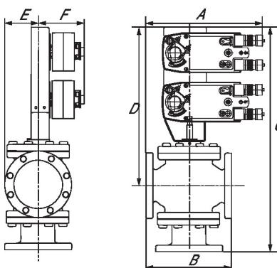
The drawing shows a front view of the actuator with dimensions E and F indicating the distance between the mounting holes. The side view shows the total height C, the distance from the base to the center of the mounting holes D, and the distance from the base to the center of the mounting holes A. Dimension B indicates the width of the actuator base.
