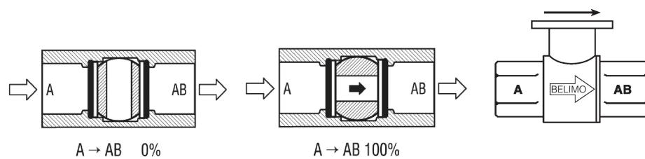
Two-way valves should be installed with the disc upstream.
