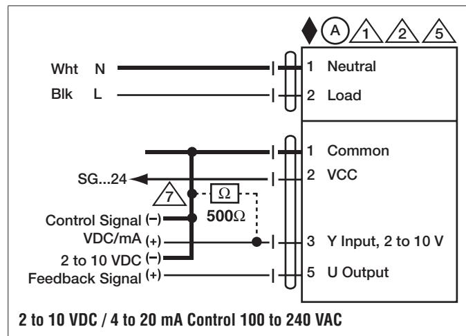
**2 to 10 VDC / 4 to 20 mA Control 100 to 240 VAC**
