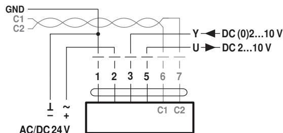
**Communication/Modbus RTU Wiring/BACnet MS/TP Wiring**
