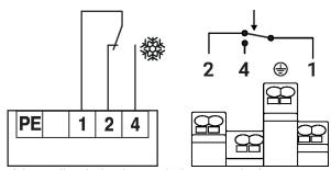
If the capillary leaks, the switch changes to the frost position.
