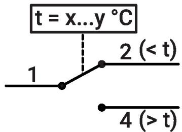
If the capillary leaks, the electrical circuit 1-2 remains permanently closed.
