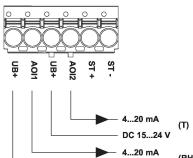
Correct temperature values are only available, when the humidity output AOI1 and both inputs UB + are connected.
