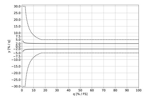
— Water ---- Water + glycol (≤60% glycol) y = Measuring accuracy q = Measured flow FS = Full scale, maximum flow
