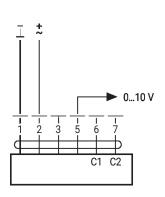
MP-Bus, supply via 3-wire connection
