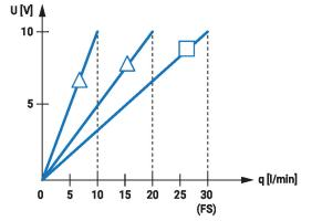
U = Output voltage q = Measured flow Δ = Alternative settings □ = Factory setting
