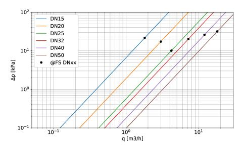
$\Delta p$  = Pressure drop q = Measured flow
