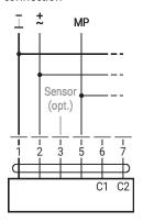
MP-Bus via 2-wire connection, local power supply
