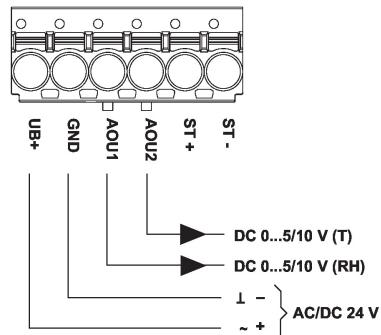
The following measuring ranges can be adjusted through the jumper settings:
