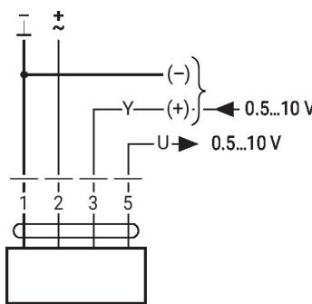
Override control (frost protection circuit)
