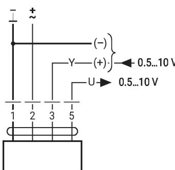
Override control (frost protection circuit)
