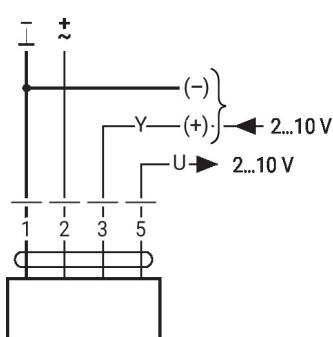
Override control (frost protection circuit)
