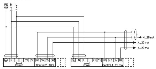
Connection BACnet MS/TP / Modbus RTU with analogue primary/secondary operation
