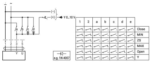
Override control and limiting with AC 24 V with rotary switch
