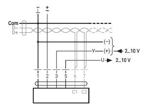
MP-Bus, supply via 3-wire connection
