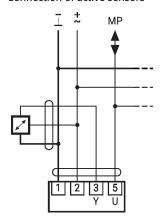
Connection of external switching contact
