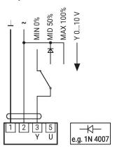
Control remotely 0...100% with positioner SG..
