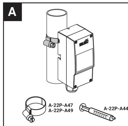
The tightening strap is included in the scope of delivery
